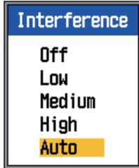
4. Use **▲** or **▼** to turn the interference rejector on or off and press the **ENTER** key.
