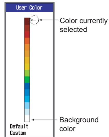
2. Press **▲** or **▼** to select the color to adjust and press the **ENTER** key. The RGB adjustment window appears.
