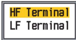
3. Use ▲ or ▼ to select a frequency terminal and press the **ENTER** key. To adjust the frequency of the transducer connected to the HF terminal, select HF terminal; select LF terminal to adjust the frequency of the transducer connected to the LF terminal.
