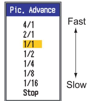
4. Use **▲** or **▼** to select picture advance speed desired and press the **ENTER** key. The fractions in the window indicate the number of scan lines produced per transmission. 1/16 is the slowest speed and 4/1 is the fastest speed. 1/16 means one scan line is produced every 16 transmissions. "Stop" freezes the display and is useful for taking a photo of the display.
