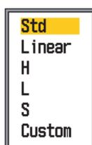
**Std:** Strong color echoes are displayed as is and weak color echoes are shown smaller, when the clutter level setting is raised.
