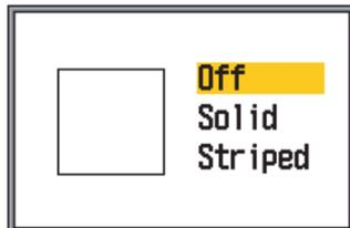
4. Use ▲ or ▼ to select Off, Solid or Striped as applicable and press the **ENTER** key. The symbol size changes with fish size as shown in the table below.
