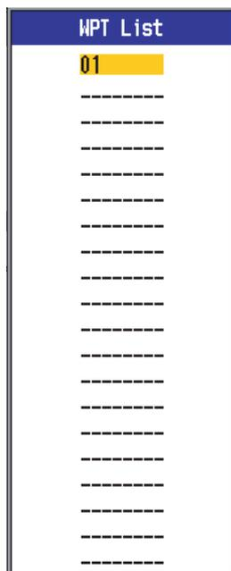
4. Use **▲** or **▼** to select an empty waypoint and press the **ENTER** key. The waypoint setting window appears, showing current position in latitude and longitude.
