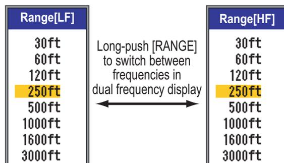
2. Push the **RANGE** control. Each press selects high or low frequency alternately.
