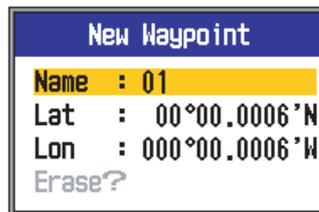
**Note 1:** When TLL or FURUNO-TLL is selected at TLL Output on the NMEA menu of the System menu, the latitude and longitude position at the cursor position is output to a chart plotter.
