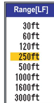
**Note:** If you are using the dual frequency display, and are set up for independent range adjustment, push the **RANGE** control to switch between low and high frequencies alternately. For details see Split Range on page 31.
