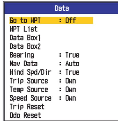
**Data Box1, Data Box2:** Turn on to display data at the upper left corner on the display. If several data items are turned on, they are displayed alternately at the interval (default: 4 s) chosen with Switching Cycle. Data other than depth and "timer" require appropriate sensor.
