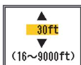
2. Use ▲ or ▼ to set range. Ranges must be set from shallow to deep, and a range can not be lower than a preceding one. The minimum and maximum ranges available are shown on the range setting window.
