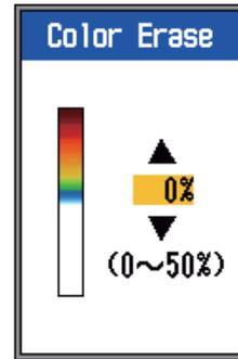
4. Use **▲** or **▼** to select the color to erase and press the **ENTER** key. The setting range is 0 to 50(%), in intervals of 5(%). The larger the setting value, the greater the number of colors that are erased.
