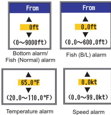
8. Use ▲ or ▼ to set starting depth, temperature or speed as appropriate and press the **ENTER** key. For Bottom and Fish (Normal), the starting depth is the range from the transducer, and for Fish (B/L), from the bottom.
